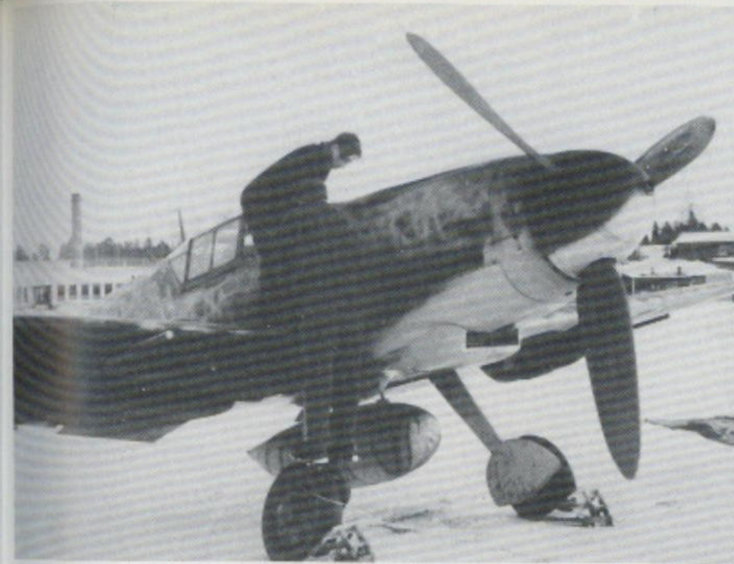
Above: First Sergeant Döring's plane of the 2./JG 300 in August of 1943, a Bf 109 G-6 with two nacelle-mounted MG 151.
