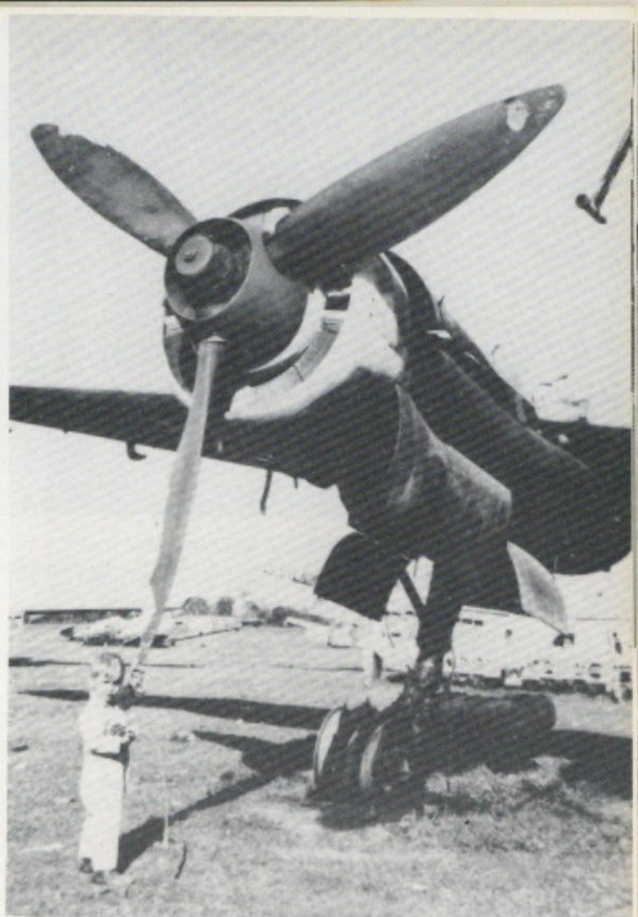
Above: Despite fire damage, this Ju 88 G-6 shows the FuG 218 V2R "Neptune" attachments and interesting details of the Jumo 213 A-1.
