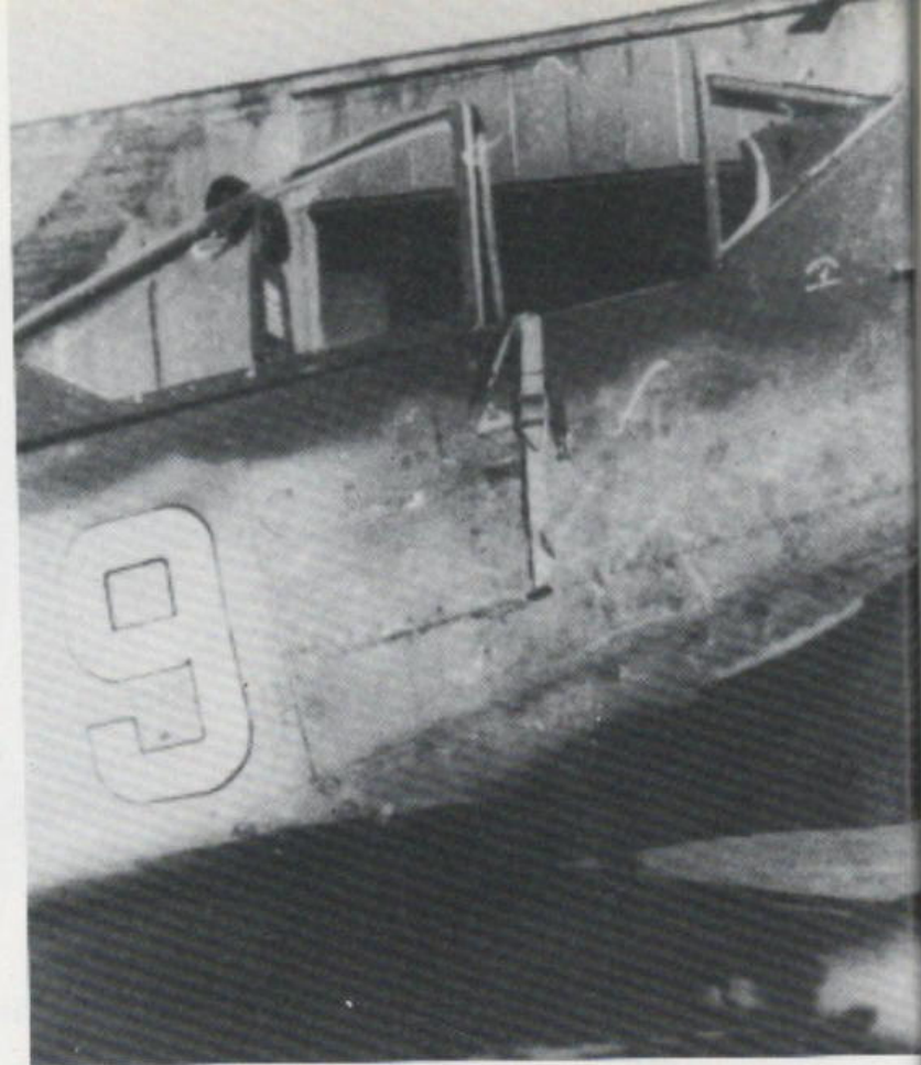
Above: The "White 9", an Fw 190 A-8 of the 1st Unit of NJG 10. A light shield was mounted over the exhaust port.
