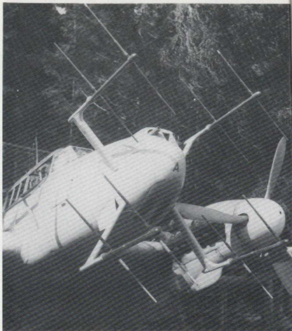
This Do 110 G-4 night fighter lies in the woods near Unterhaching and shows damage to its radiator. Note the two MK 108 as bow armament and the antenna dipoles painted in warning colors.
