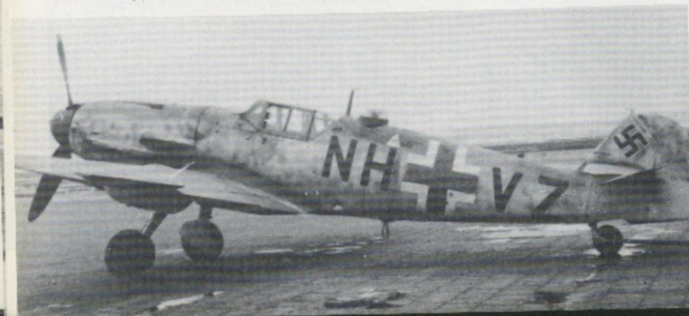
Below: Another model with FuG 350 "Naxos Z" system housed under the glass canopy.
