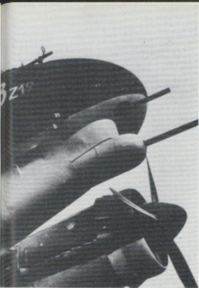
Above: Bow of model plane Ju 88 V19, also called Z19 (factory number 0373), after an additional 20-mm gun had been installed.
