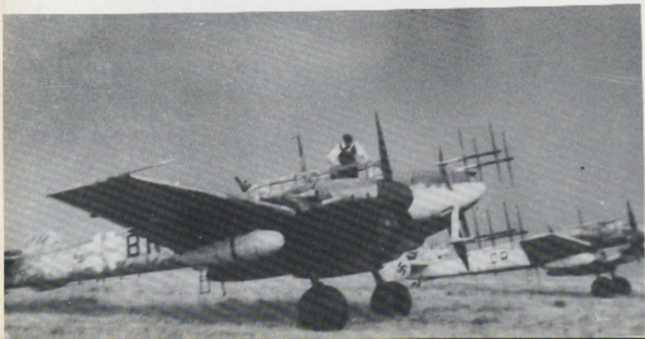
A Bf 110 G-4 in the winter of 1945, with the same equipment, including FuG 212 and 220.
