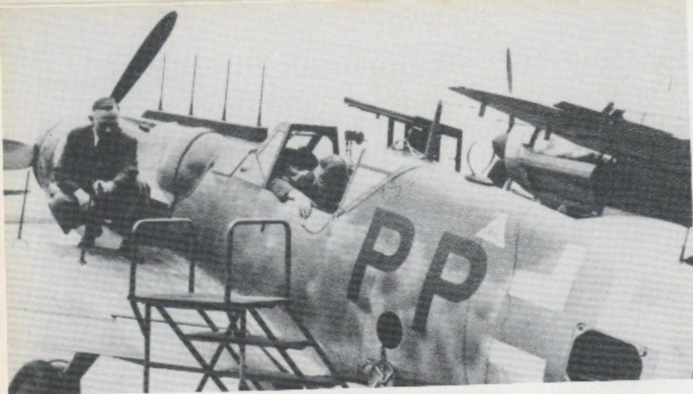
Above: The experimentally reequipped Bf 109 G-6/N with the antennae of the FuG 217 "Neptune" system.
