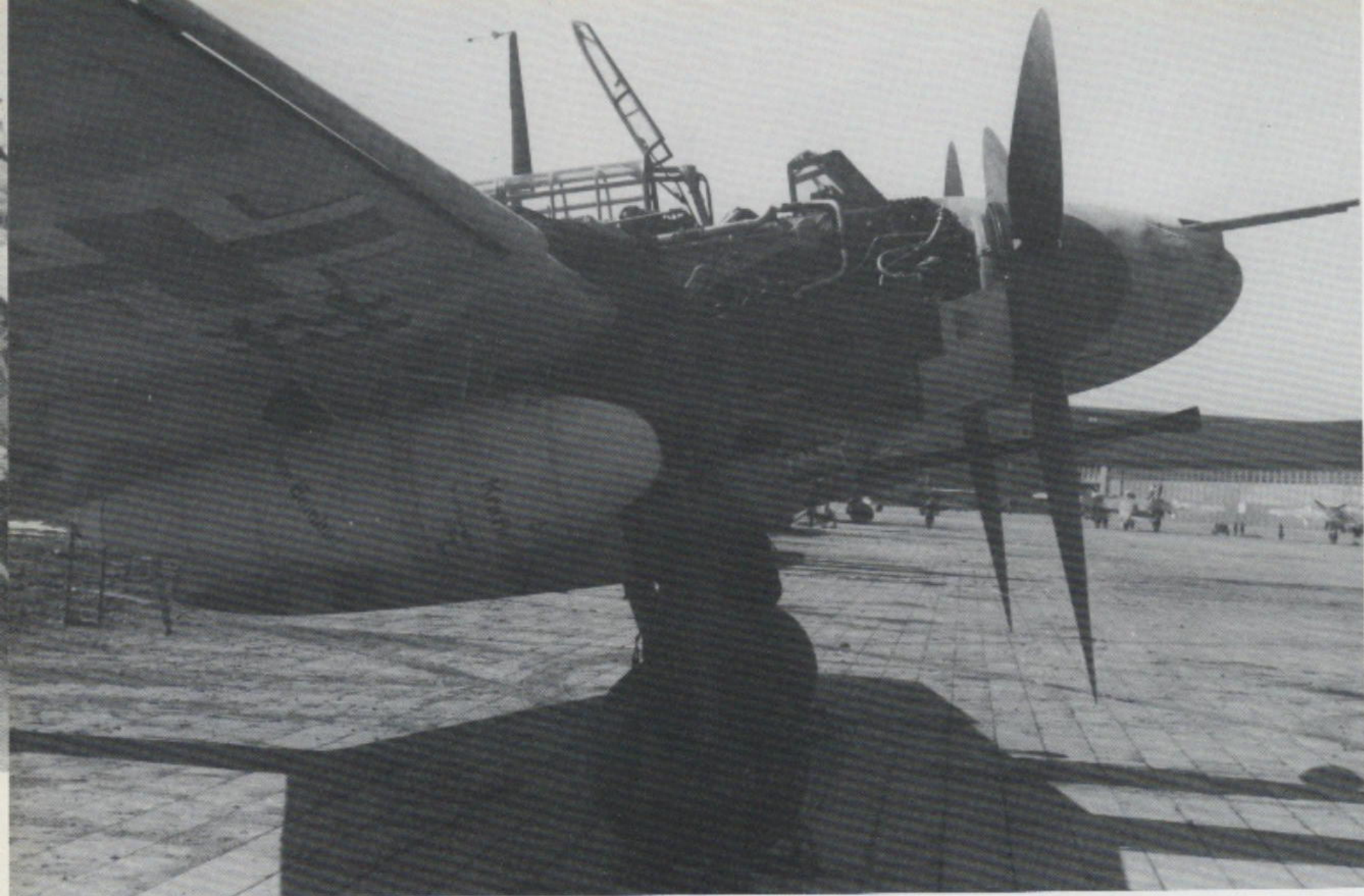
A heavy night fighter of the Bf 110 G-1 type, with two MG 151/20 instead of two MK 108 at the bow. Under the fuselage there is also a 37-mm cannon.
